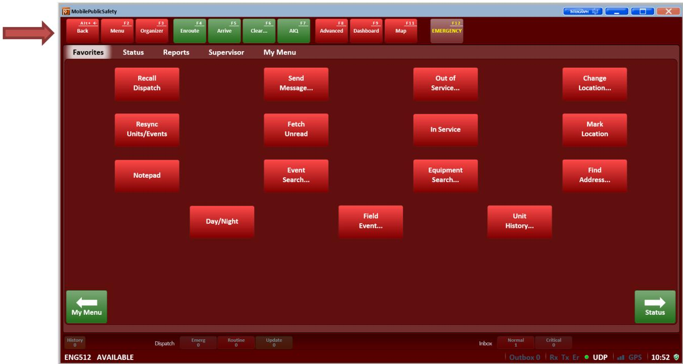
The Toolbar is located at the top of all of the MPS screens. The toolbar functions are also associated with the “F” or function keys on your keyboard. These icons will assist you in rapidly navigating the MPS software.
